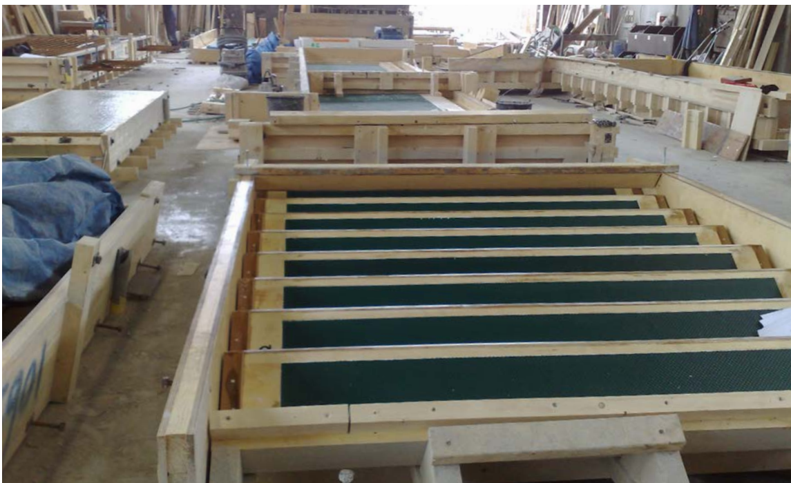
Examples of a GIAN® pattern mat glued into a wooden concrete mould.
