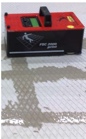
A wet concrete imprint from the GIAN®1 diamond is being tested with the FSC 2000 print.
