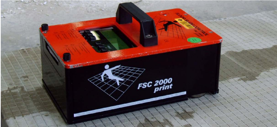
The FSC 2000 print is a manageable machine to measure frictional resistance on location.
