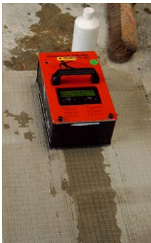
The FSC 2000 print tests a wet concrete element with a GIAN® 2s concrete pattern.
